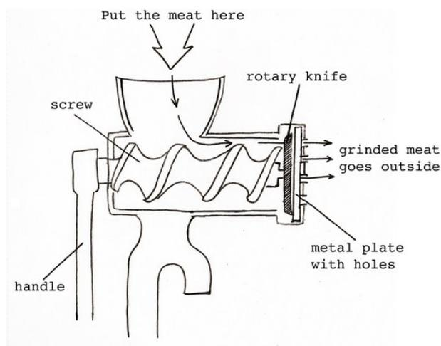
Fig. 2. Meat grinding process
